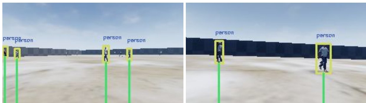
Figure 16: Yolo closeness metric in the custom environment with pedestrians
